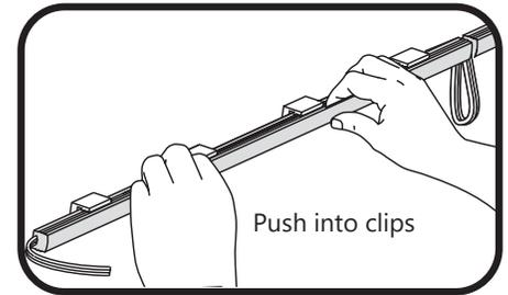
3 Push each 16 in. (406mm) light engine segment into the clips. Fold loose wires behind light engines. Do not stretch light engines.
