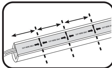
**2** Using the light guide final length, measure out the necessary length of Contour LED light engine to match. If required, using a sharp cutting tool, cut wire loops between sections or through light engine (refer to the Cutting Resolution Table on page 2).
