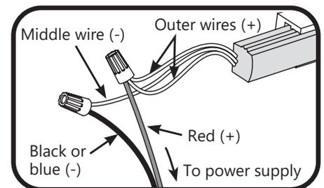
9 Connect the two outer wires (+) from the LED strip to the red wire (+) of the power supply. Connect the middle wire (-) from the LED strip to the black or blue wire (-) of the power supply. Grounding and bonding must be done in accordance with National Electrical Code (Article 600). See power supply instructions.
