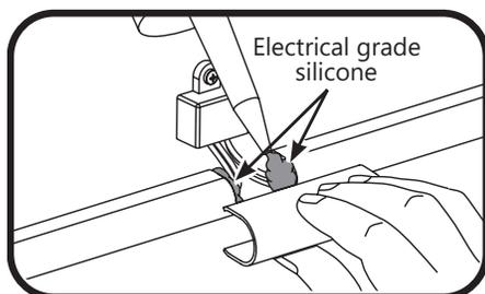
**13** Linear: At each gap between sections, apply silicone on both sides to secure light guide connector. Snap on a light guide connector.
