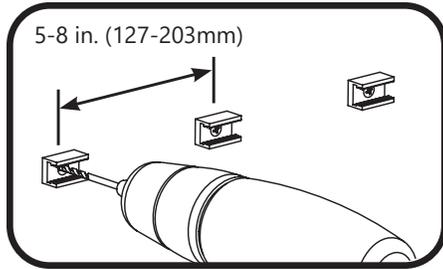
1 Install a mounting clip, using #6 (M2) counter sink screws, every 5–8 inches (127–203mm) on center until the end of the run is reached.
