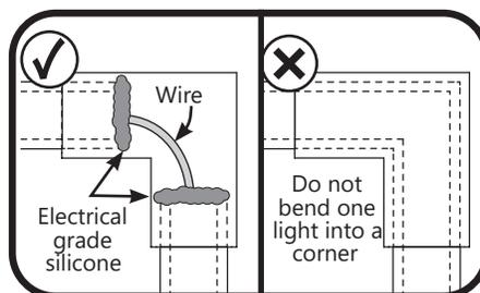
**14** Corner: For all corners (planar, inside, outside) apply silicone on both sides to secure light guide corners. Snap on corner. Follow Steps 8-10 if wires are cut.
