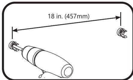
**1** Install a minimum of one clip per 18 in. (457mm) using #10 (M4) screws.
