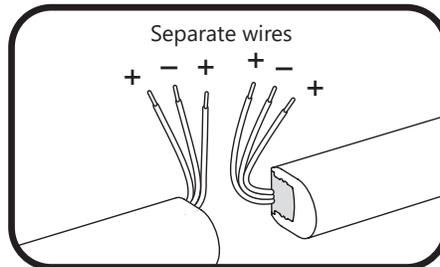
**8** To connect two light engines separate wires and identify outer conductors as positive (+) and middle conductors as negative (-). Strip ends back 0.5 in. (13mm).
