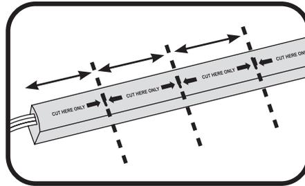
2 Using the light engine final length, measure out the necessary length of Contour light engine. If required, using a sharp cutting tool, cut wire loops between sections or through light engine.
