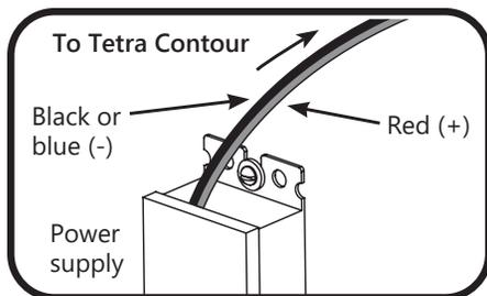
7 Run a wire from the power supply to a section of Tetra® Contour. Power supply connection must be completed in an acceptable UL/ NEMA enclosure. Power supply loading is described in the power supply installation instructions.
