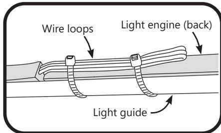
**7** Wires between light guide segments can be folded behind the light guide and attached with clear zip ties. Zip ties should wrap around outside light guide.
