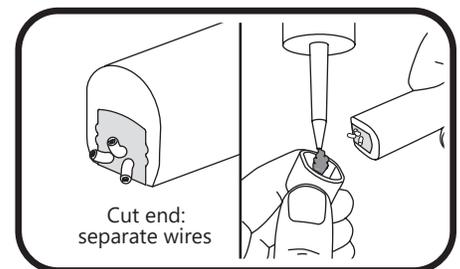
**12** For uncut end, fold wire over Tetra® Contour. Fill the end cap with silicone and push cap on the end to secure. Clean excess silicone.
