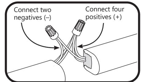
**9** Use twist-on wire connectors to join wires together.
