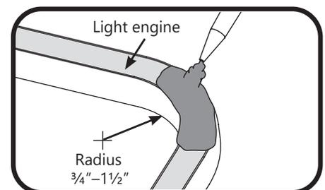
**15** Bends having an inside radius 1 1/2" or smaller must have electrical grade silicone applied directly to the light engine across the bend.
