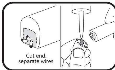
**11** For cut end, manually untwist and separate wires to avoid shorts. Fill cap with electrical grade silicone and push cap on the end to seal. Clean excess silicone.
