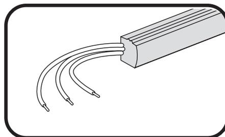
8 Separate wires and identify outer conductors as positive (+) and middle conductor as negative (-). Strip ends back 0.5 in. (13mm).
